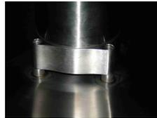
**Step (4):** Align each tier collar over corresponding placement grooves on the cylinder, starting with the largest tier, then the medium tier and then the smallest tier.
